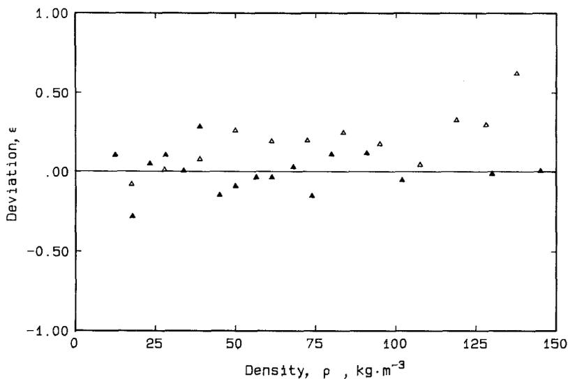
Fig. 1. The deviations of check measurements of the thermal conductivity of argon at 308.15 K from the correlation of Eq.(1). (▲) This work; (△) Ref. 1.  $\epsilon = [(\lambda_{\text{expt}} - \lambda_{\text{corr}})/\lambda_{\text{corr}}] \times 100\%$ .
