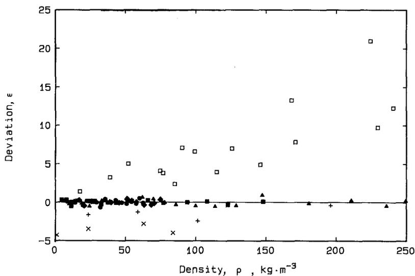
Fig. 2. Deviations of measurements of the thermal conductivity of ethylene from the present correlation.  $\epsilon = [(\lambda_{\text{expt}} - \lambda_{\text{corr}})/\lambda_{\text{corr}}] \times 100\%$ . This work: (▲) 308.15 K; (■) 333.15 K; (◆) 371.15 K; (●) 425.65 K. Lenoir and Comings [12]: (+) 314.2 K; (x) 340.3 K. Prasad and Venart [10]: (□) 299 K.
