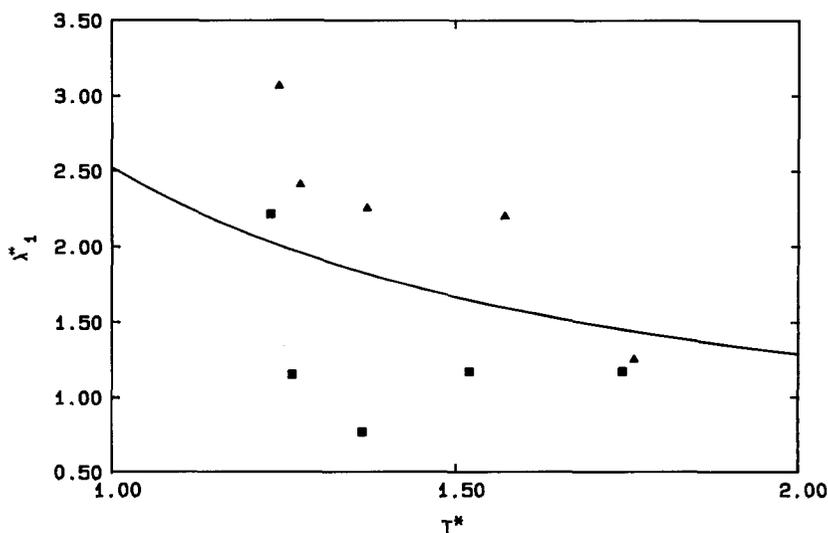
Fig. 6. Reduced first density coefficients for ethylene (■) and ethane (▲).
