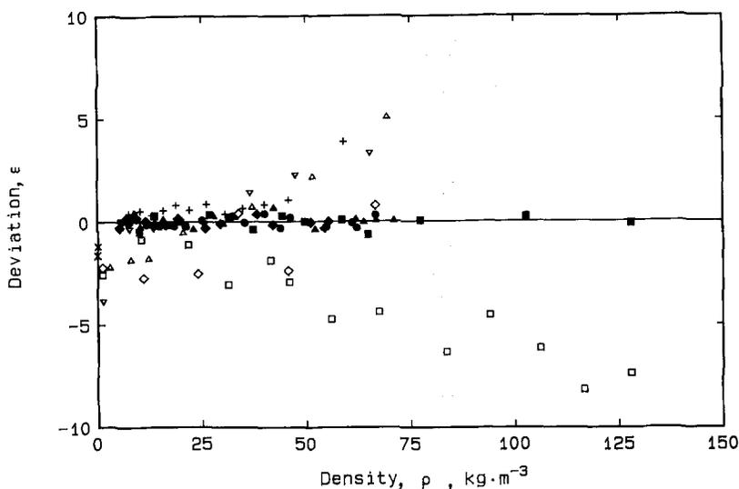
Fig. 3. Deviations of measurements of the thermal conductivity of ethane from the present correlation.  $\varepsilon = [(\lambda_{\text{expt}} - \lambda_{\text{corr}}) / \lambda_{\text{corr}}] \times 100\%$ . This work: (▲) 308.15 K; (■) 331.65 K; (◆) 380.15 K; (●) 425.65 K. Roder [17]: (△) 305 K; (▽) 312 K. Tufeu *et al.* [16]: (x) 312 K. Lenoir *et al.* [15]: (□) 329.8 K; (◇) 315 K. Fleeter *et al.* [14]: (+) 300.6 K.
