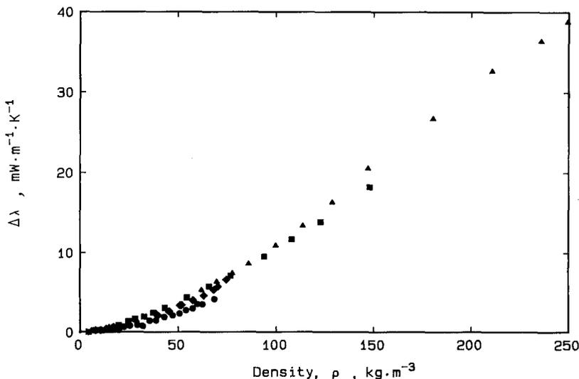
Fig. 4. The excess thermal conductivity of ethylene. (▲) 308.15 K; (■) 333.15 K; (◆) 371.15 K; (●) 425.65 K.
