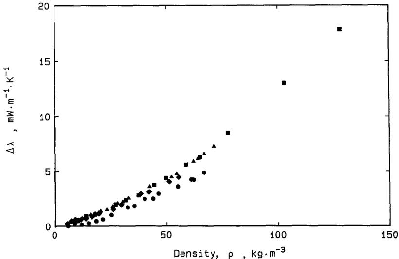
Fig. 5. The excess thermal conductivity of ethane. (▲) 308.15 K; (■) 331.65 K; (◆) 380.15 K; (●) 425.65 K.
